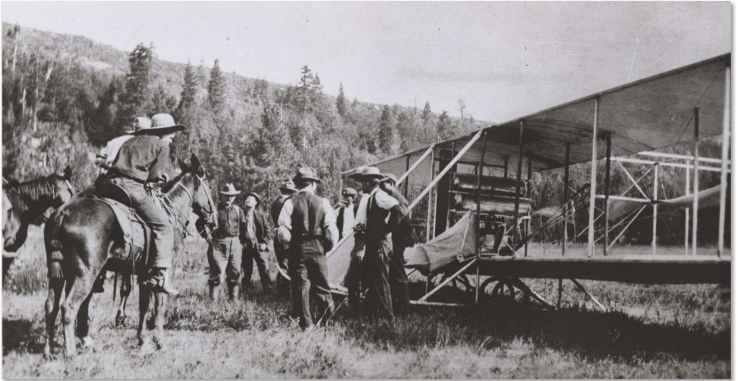
Robert Fowler's biplane, built by the Wright Brothers, 1911. After Fowler crashed northeast of Colfax during his attempt to fly from San Francisco to Jacksonville, Florida in less than 30 days, his plane was repaired in Colfax, with additional work performed in Grass Valley. It utilized a 30-horsepower engine from the Cole Motor Car Company. From the online collection of the California State Library.
